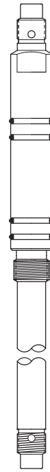
Feedthru seals in the tubing hanger and the adapter flange with O-rings and is held in place with threads on the metal shell.
