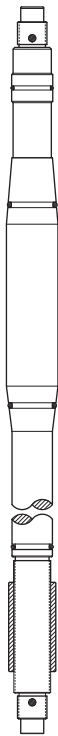
Feedthru uses metal-to-metal seals backed up with O-rings and is held in place with a retaining nut pulling against a machined shoulder on the metal shell.
