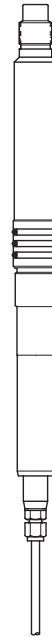
Instrument packer feedthru has factory molded lower cable and a crossover adapter (not shown) to fit the top end of the packer. Splice assemblies are also available to join the cable from the packer feedthru to the I-wire cable below the packer.
